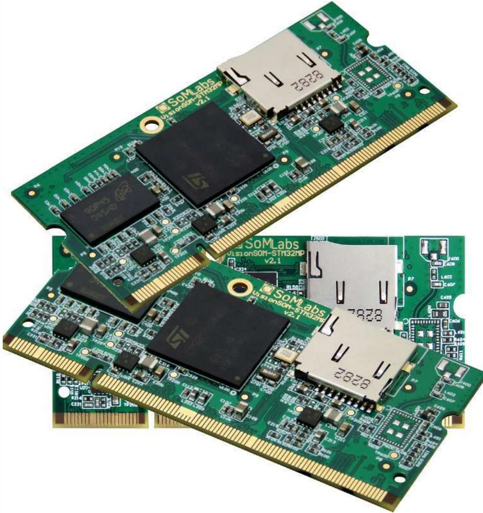
The VisionSOM-STM32MP1 family is a SODIMM-sized SoM based on the STMicroelectronics STM32MP1 application processor which features an advanced implementation of a single or dual ARM Cortex-A7 cores (at speed up to 650MHz) and ARM Cortex-M4 core (at speed up to 209MHz) as well as a 3D Graphics Processing Unit (GPU) Open GL 2.0 ES compatible.
